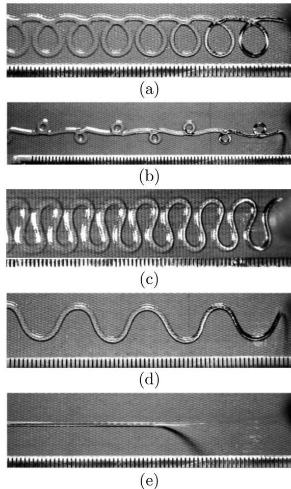
FIG. 4. “Main sequence” of stitch patterns in the FMSM at increasing speed of the belt. (a) coils; (b) “one-by-one” (c) bunched-up meanders or “braiding”; (d) meanders; and (e) catenary. Photographs courtesy of J. R. Lister.
