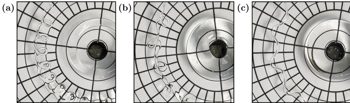
**FIG. 6.** Asymmetric traces in the R-FMSM setup for the flow rate  $Q = 2$  ml/min, fall height  $H = 5$  cm, and at the radial distance  $R = 3$  cm, at three different angular speeds. (a) translated coils; (b) “one-by-one”; (c) meanders. The working fluid is silicone oil with  $\nu = 0.03$  m<sup>2</sup>/s. Circular markings, separated by 0.5 cm, provide scale. Pictures taken from the forthcoming Ref. 13.
