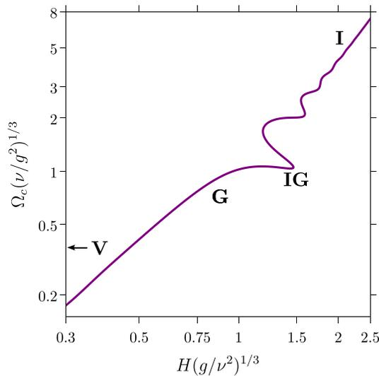
FIG. 2. Dimensionless coiling frequency  $\Omega_c(\nu/g^2)^{1/3}$  as a function of dimensionless fall height  $H(g/\nu^2)^{1/3}$  for the flow rate  $Q(g/\nu^5)^{1/3} = 0.025$  indicating the coiling regimes useful for culinary flows.<sup>13</sup>
