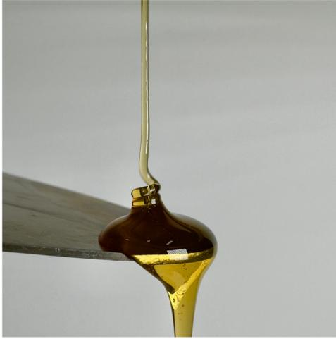
FIG. 1. Coiling of natural honey filament on a spoon, at a flow rate of  $Q \sim 1 \text{ ml/s}$ , pouring from a height of  $H \sim 10 \text{ cm}$ .
